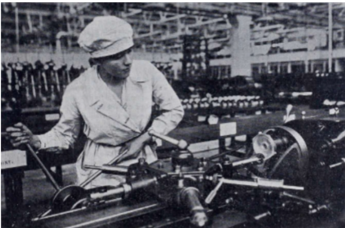
Figure 1: Cover photo of TWE's third issue showing a woman boring the body of a magneto on a No. 4 Herbert Turret Lathe (Haslett 1920, 21)
